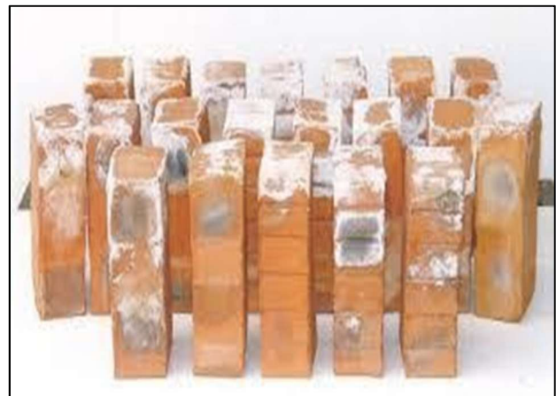
Fig.11.2 Efflorescence observed after immersion
