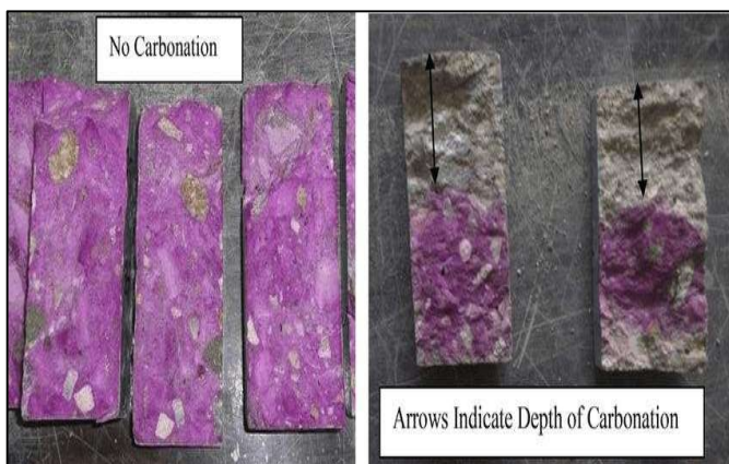
(c) Measurement of depth of carbonation.
