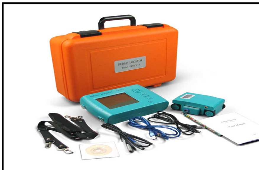
Figure No. 6: Rebar Locator with accessories
